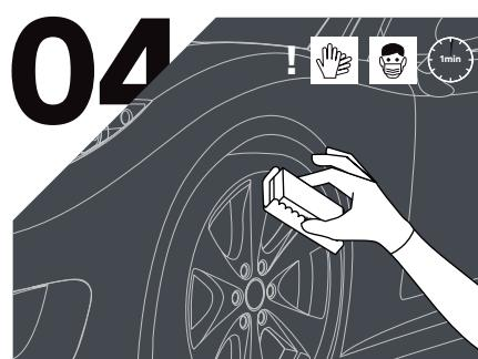
Apply nice and evenly as you go. Do not try to spread too thin but be sure to work to an even coat in the first minute before moving to the next overlapping area.
