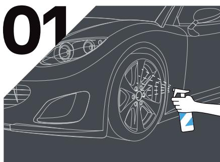
Wipe surface with **Carpro Eraser**, wipe dry, and then allow evaporation 20 min before applying.
